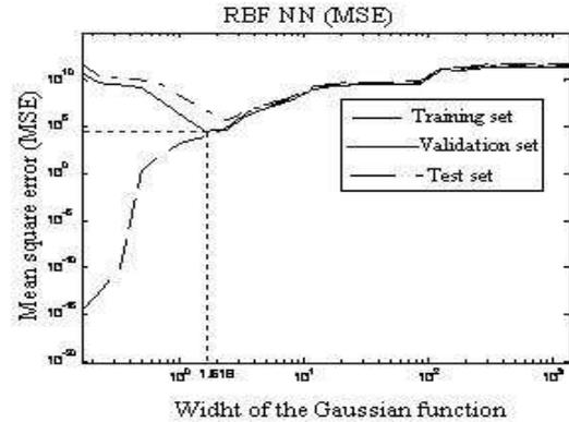
Figure 7: The evolution Mean Square Error on the tree sets for the RBF NN
