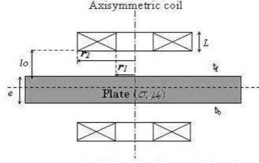
**Figure 1:** Geometry and dimensions of the solenoids used in method A-O for motionless sheets
