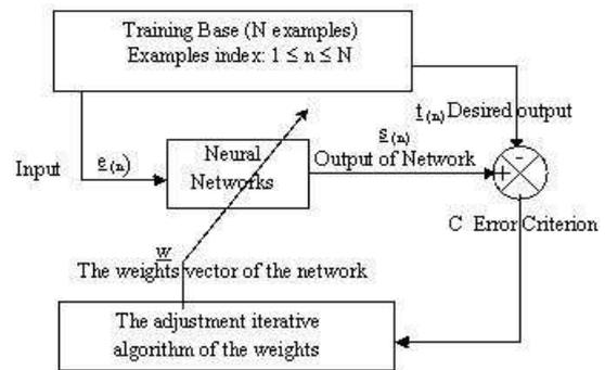
Figure 4: The weights adjustment of the MLP NN
