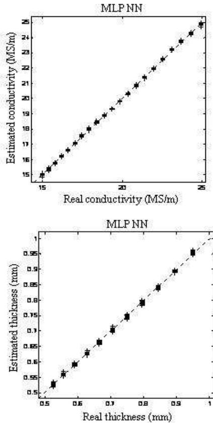
**Figure 9:** The evaluation vs real values of the conductivity and the thickness on the test set (+) per MLP NN
