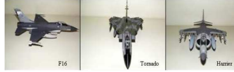
Figure 3: Scale reduced aircraft models used in the anechoic chamber
