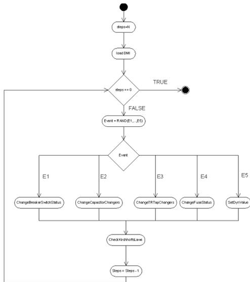
**Figure 1:** The UML activity diagram for the profile 1 (changing dynamic data)
