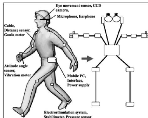
Figure 7: Wearable sensory devices used in Wearable Robotics.
