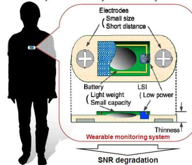
Figure 3: Monitoring system restrictions wearable.
