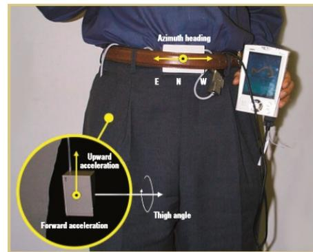
Figure 4: Implementation of wearable in Motion Recognition
